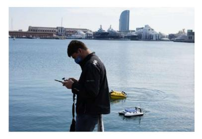
During the operation, GPASEABOTS deploy 2 USV equipped with different instrumentation each with the objective of providing a complete service for the needs of a port as large and important as the Port of Barcelona.
