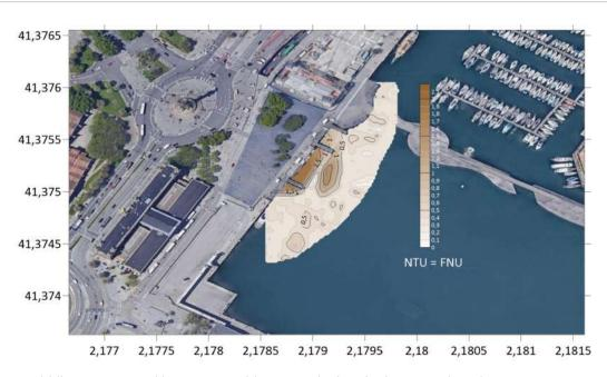
Turbidity measurated by WIMO Multiparametrical probe integrated on the SB 100 PRO.
