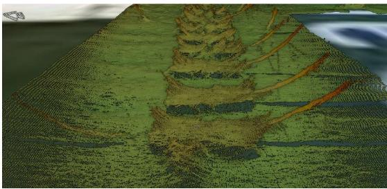
This tool is also capable of identifying the anchoring chains of vessels. As an example, this image of the raw data of this case.
